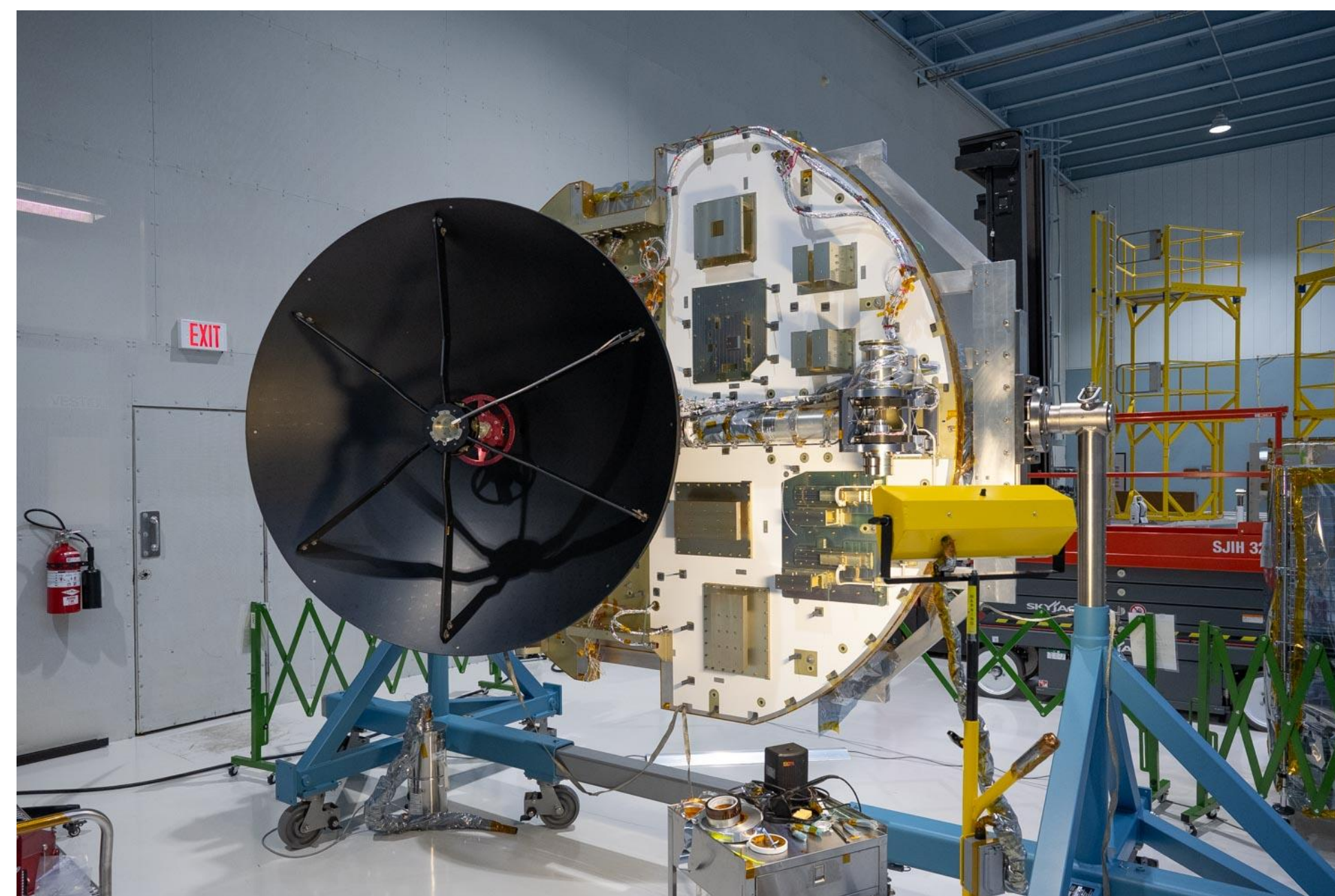
Fig. 1: Roman Space Telescope High Gain Antenna System Image Credit: NASA
