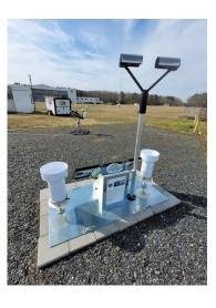
PIERS+ site including a PARSIVEL disdrometer and two tipping bucket gauges on the same olatform
