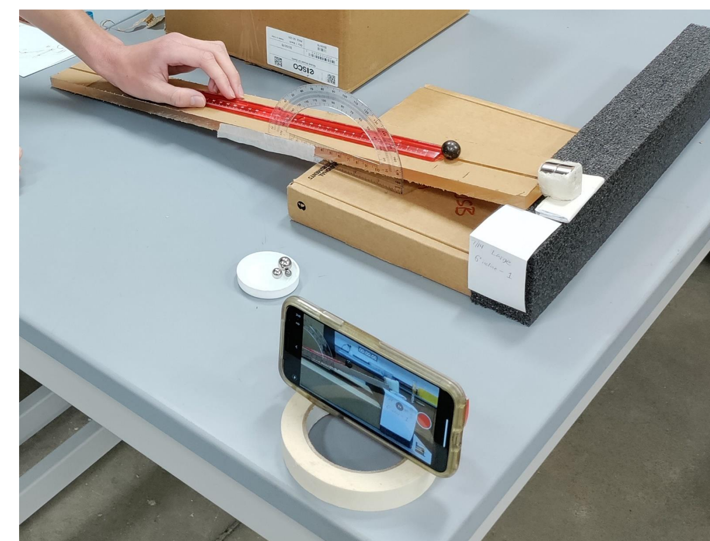
Fig. 4: using a smartphone to record the motion of the ball in slow motion so that its position, speed and acceleration can be determined with a Tracker app
