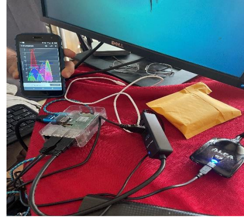
Figure 1 shows a Raspberry Pi computer board set up to act as a Wifi access point
